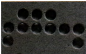
Figure 3: A small section of a Jacquard card
