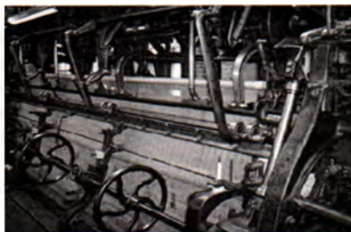
Figure 2 An operating Leavers machines. La Cité de la Dentelle 2009
