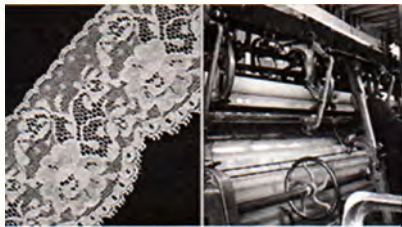
Cluny lace is made using traditional Leavers and Jacquard machines.
