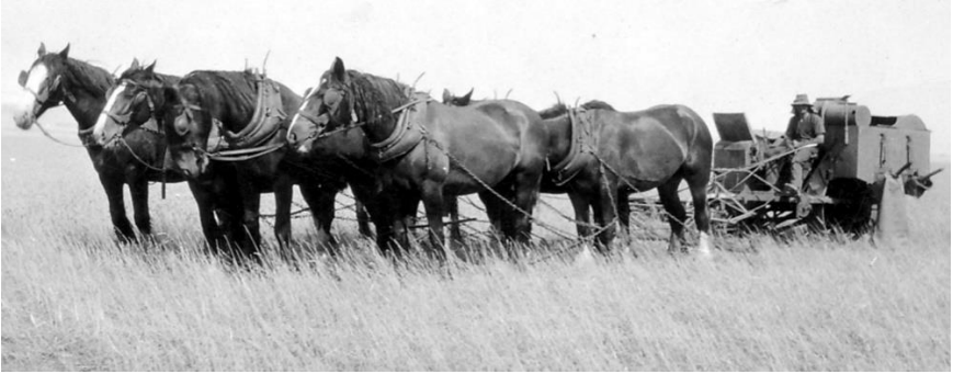
Longmire Team of Clydesdales hitched to a ground-driven wheat harvester with an Australian Front (long combs - Sunshine Make)
